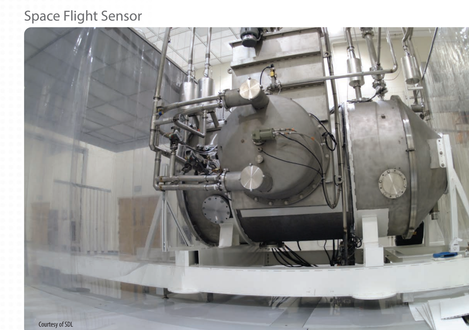
TVAC chamber to simulate the space environment Cryogenic operating pressure: \sim 10^{-4} Torr LH 2 shroud provides low background
