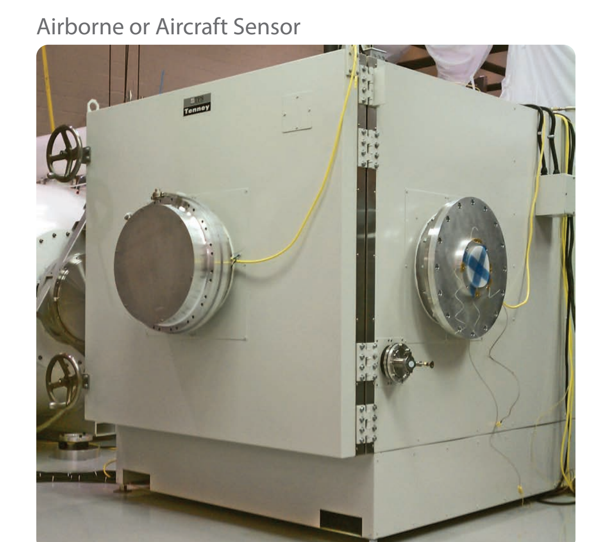
Altitude simulation: (0 to 100,000 ft.) Temperatures: -60°C to 125°C Pressure: Ambient to \sim 10 Torr
