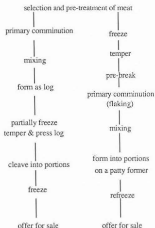
Fig. 1. Two common methods of manufacture of restructured meat products. The sequence of operations on the right is followed by most UK manufacturers; the scheme on the left has been followed by most of the literature on the subject.
