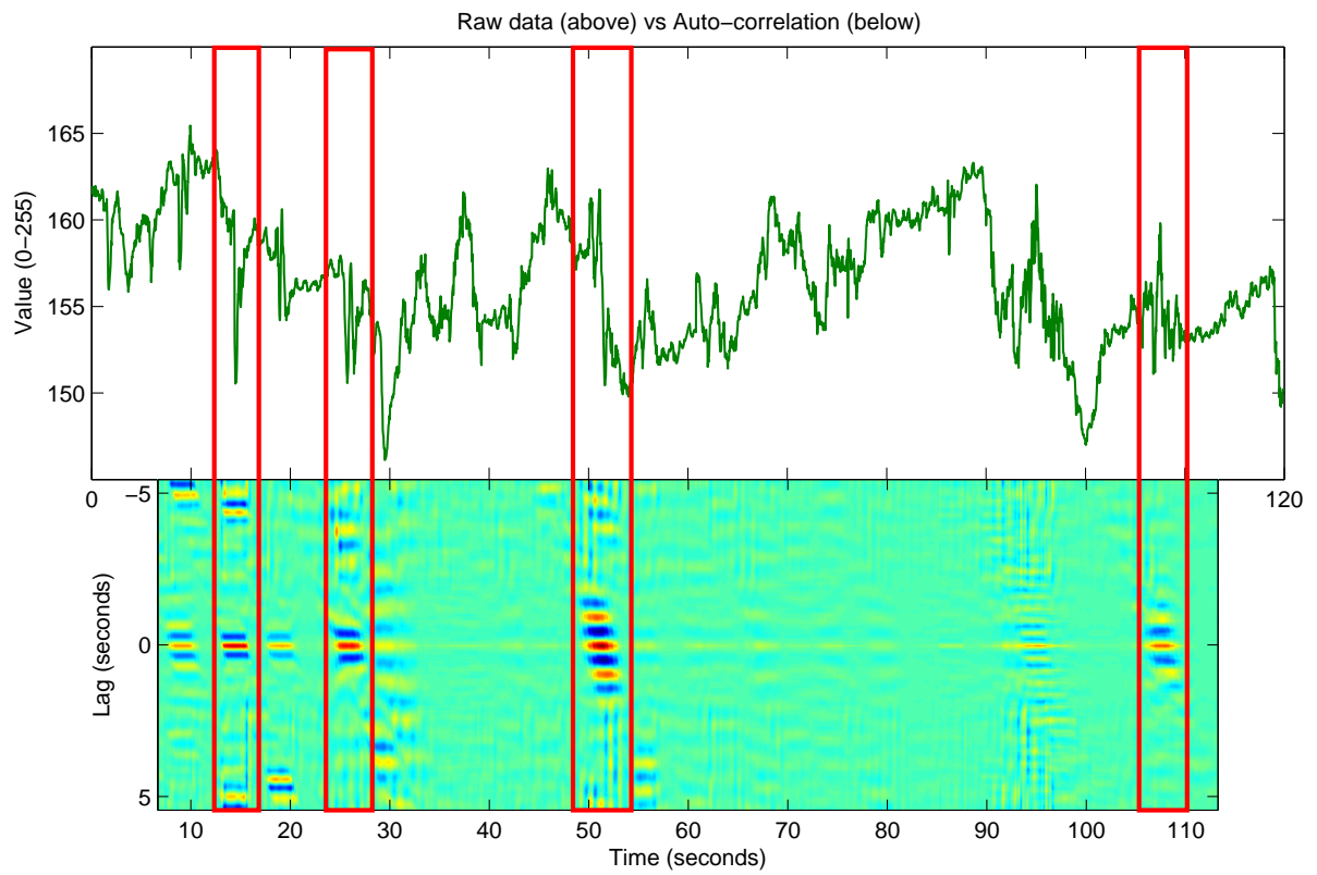
Fig. 3.5: Comparing the transient effects of the time-domain data to the large auto-correlation samples. The red boxes highlight the artifacts of interest.
