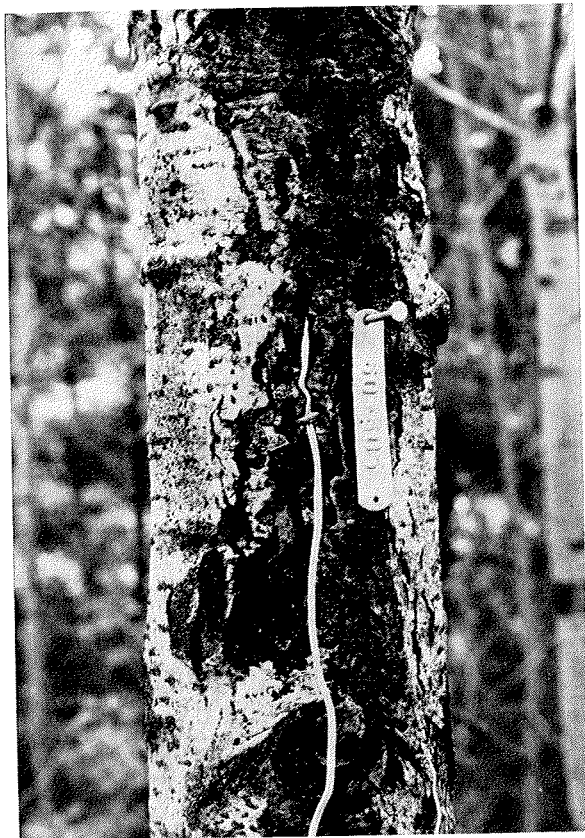
Fig. 1. Copper-constantan thermocouple embedded in the healthy bark of an aspen tree just below a Hypoxylon canker. The thermocouple junction is approximately 5 cm above the point at which the lead enters the bark.
