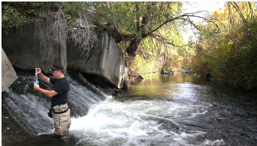
Photo 2. J. Fuller filtering water samples from the effluent of the possible point source (White's Trout Farm). The periphyton sample was scraped from the cement surface of the effluent channel. This site is located ca. 20 meters above Station 5.
