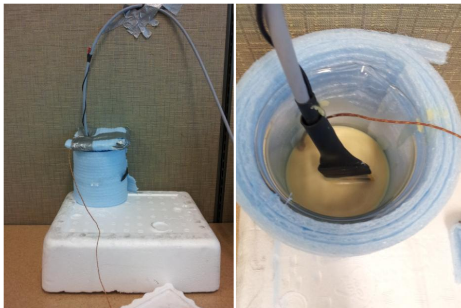
Figure 5: HotDisk® Experimental Set-up for Measuring Liquid Thermal Properties
