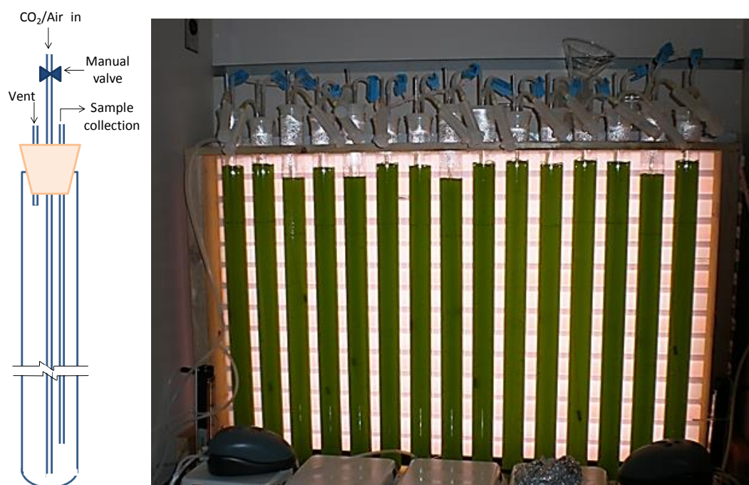
Figure 2. Airlift tube PBR schematic and set-up
