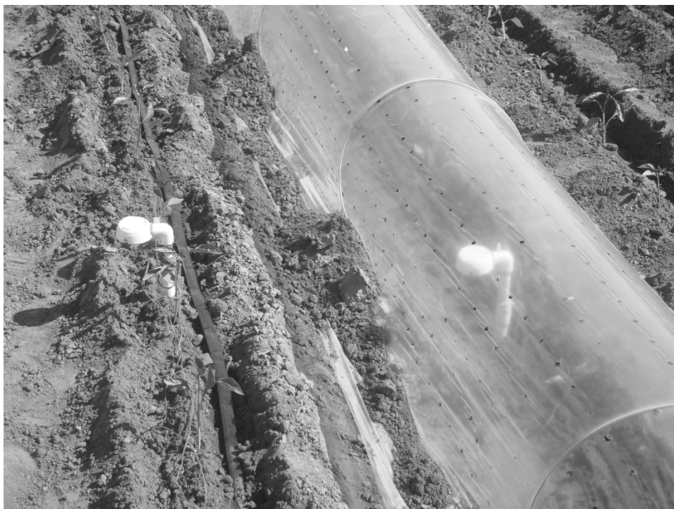
Figure. 2.2. Air and soil temperature sensors location outside and under the low tunnel in 2013.
