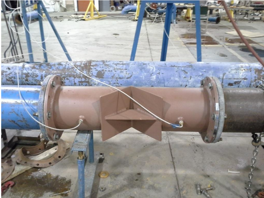
Fig. 10. Wedge flow meter installation.
