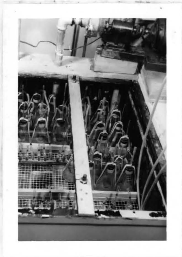
Figure 14. Partially filled bath showing the capillaries connected to the air manifolds and to the samples
