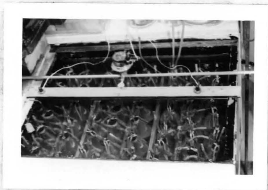
Figure 17. Apparatus for moisture, temperature and aeration control during incubation of samples
