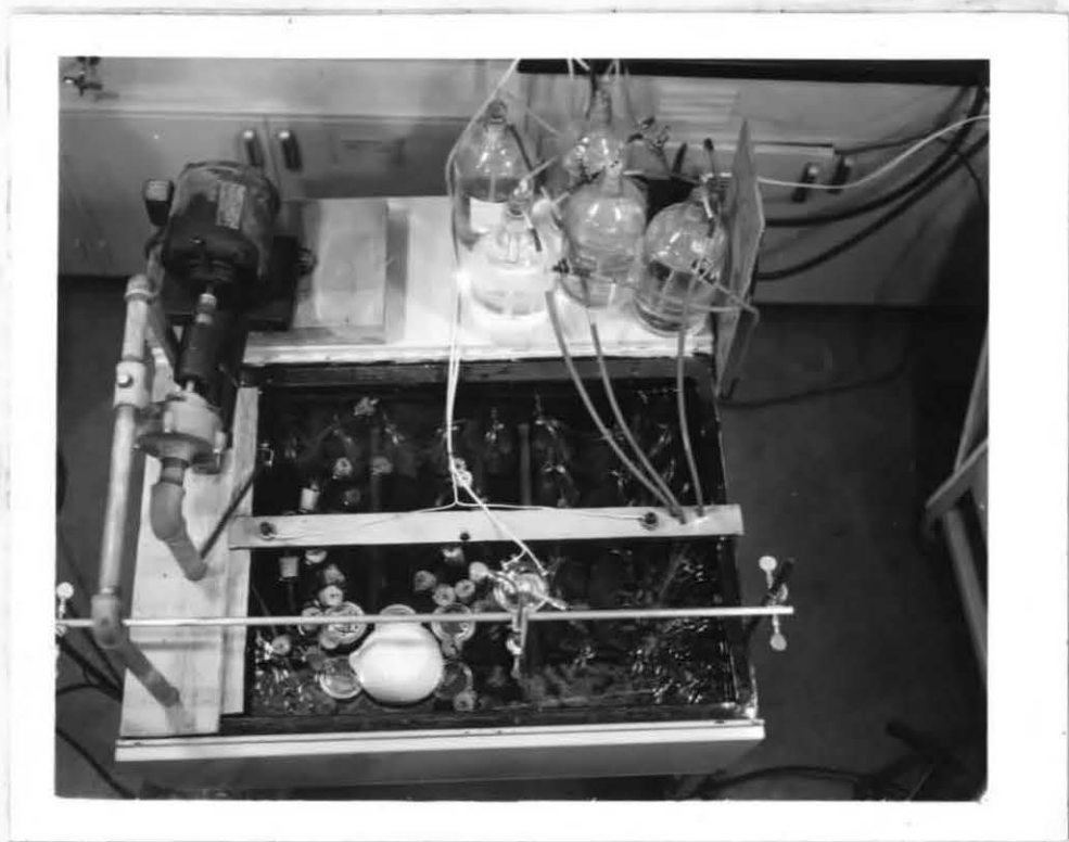
Figure 18. Apparatus for moisture, temperature and aeration control during incubation after some of the samples have been removed
