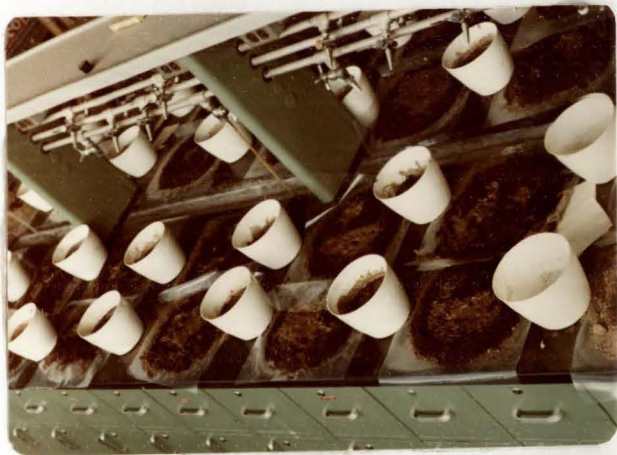
Figure 3. A few of the 750 plus samples as they appeared after mud was ponded on the soil and air dried prior to mixing.
