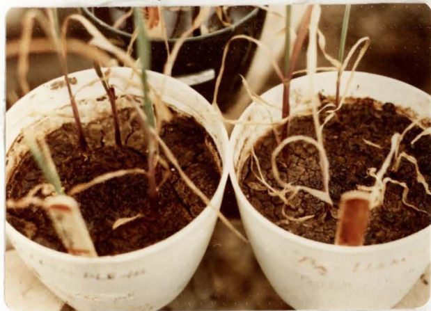
Figure 5. A close-up view of soil crusting in mixtures using lignite lignosulfonate sodium muds (LLSM). Note the plants that have died and dried up.
