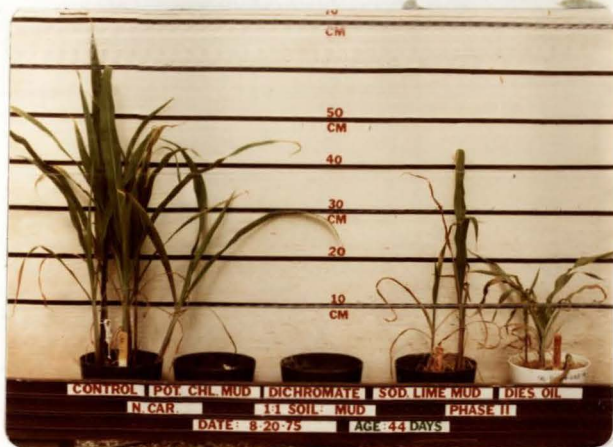
Figure 38. Green bean growth in 1:1 soil-mud mixtures of North Carolina soil with potassium chloride mud, dichromate mud, high pH lime mud, and diesel oil emulsion mud. No other treatment; no leaching.
