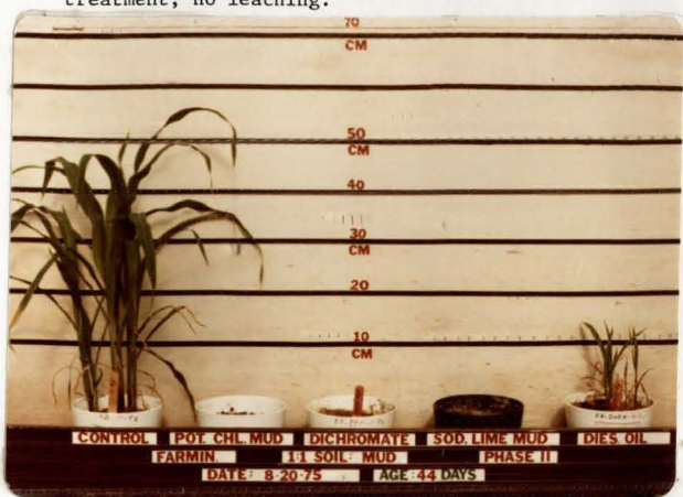
Figure 41. Sweet corn growth in 1:1 soil-mud mixtures of (Kidman) Farmington soil with potassium chloride mud, dichromate mud, high pH lime mud, and diesel oil emulsion mud. No other treatment; no leaching.
