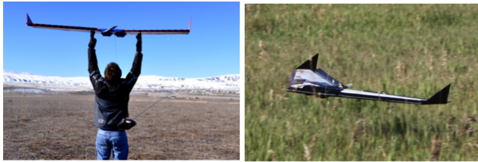
Fig. 2.3: AggieAir flying wing bungee launch and skid landing.
