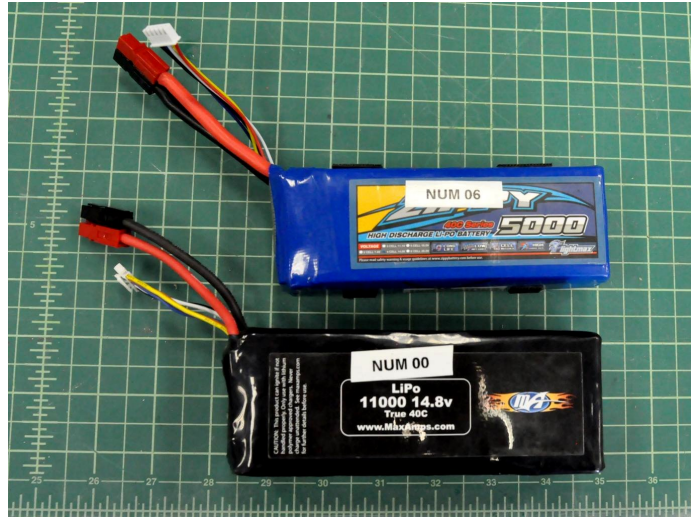
Fig. 7.10: Zippy 5000mAh 40C 4-cell battery (above); MaxAmps 11000mAh 40C 4-cell LiPo battery (below).
