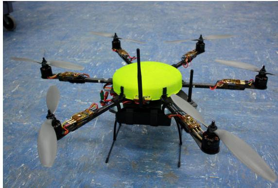
Fig. 2.7: AggieAir Multirotor Platform (Hexarotor), ready for flight.
