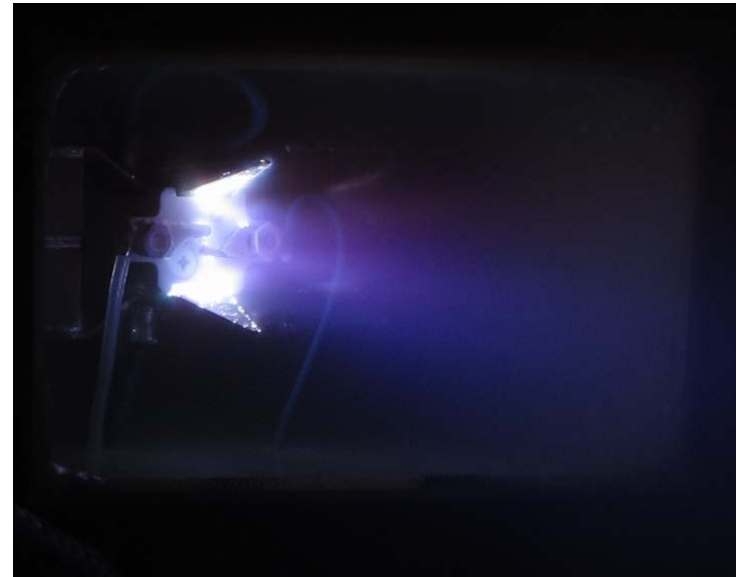
Thruster operating 900 V. Long exposure photographs over a single discharge.
