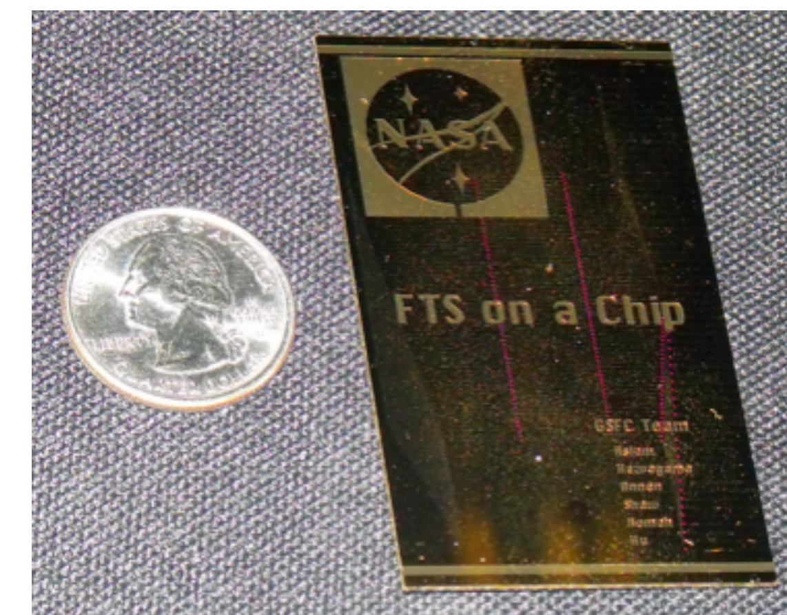
Figure 1. Image of an assembled micro-FTS chip containing multiple Mach-Zehnder waveguide pairs with a quarter shown for scale. Several chips could be stacked together to create a device capable of sampling a wider spectral range.
