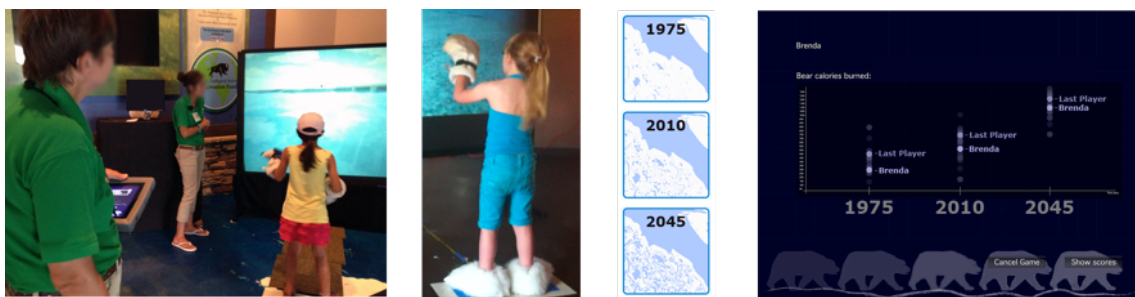
Figure 10. On the left, Paws in use in the Brookfield Zoo. Middle left, a player wears plush gloves containing motion sensors, and stands on a pressure-sensitive plate, to swim and walk, respectively, through three different decades of a simulated arctic environment (maps, middle right). The right image depicts the graphical representation of visitors' performances across the decade, with the most recent two visitors' data highlighted.
