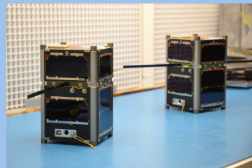
Left: 2 FIREBIRD spacecraft fully assembled with antenna deployed. The top 1/3 of the spacecraft contains FIRE (the instrument, built at UNH) while the bottom 2/3 is BIRD, built by MSU.
