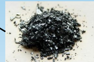
320cc Iodine Propellant Stored as Solid Crystals
