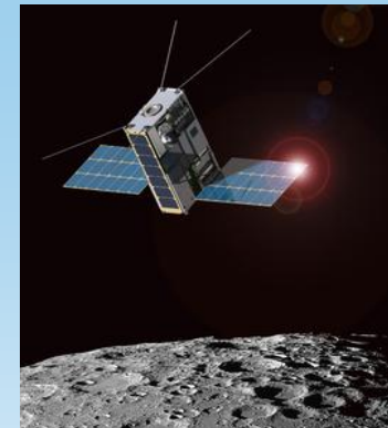
The Upcoming “Lunar IceCube” Mission is Based on the 6U LunarCube Platform
