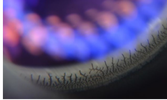
Figure 10: Delamination in the adhesive used in the element 3 doublet of the Custom lens.
