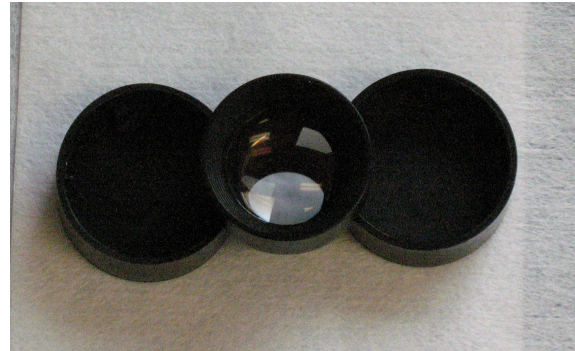
Figure 2: Vignetting observed by viewing back-lit lens from off-angle (notice the bright circle is interrupted by the lens edge.)
