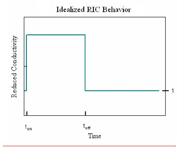
In an idealized model, when incident radiation begins at ton, the conductivity is enhanced instantaneously. Once the radiation ceases, the enhancement disappears instantaneously.
