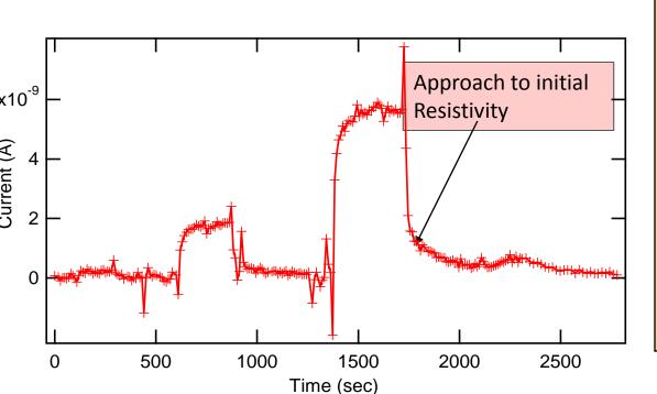
Resistivity of an irradiated Kapton E sample was tested 16 days afte radiation exposure, to look for lon term effects. No electric field had been applied to this sample durin irradiation. Using the constar voltage method, we determine the resistivity at several electri field strengths (table at right). Th average measured resistivity was full order of magnitude less that that exhibited by unexpose Kapton E.
