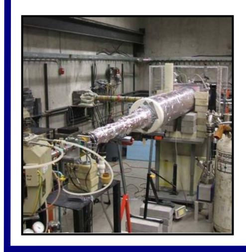
The figure to the left shows our assembly at the Idaho Accelerator Center. We employed a 25 MeV LINAC accelerator to bombard our samples with high-energy electrons at 4 MeV at a dose rate of 0.01 to 10 Rad/s.
