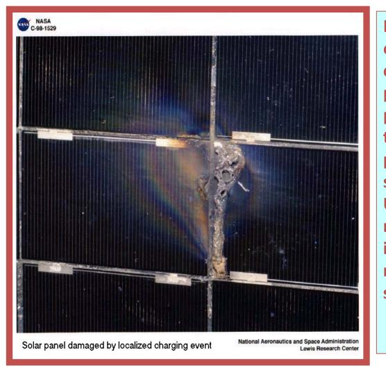
Interaction with the plasma environment induces spacecraft Electron, ion, and charge-induced potentials can result in arcing, thus damaging electronics, solar or other spacecraft components. **Understanding** how charge migration and dissipation occurs effects of spacecraft charging.
