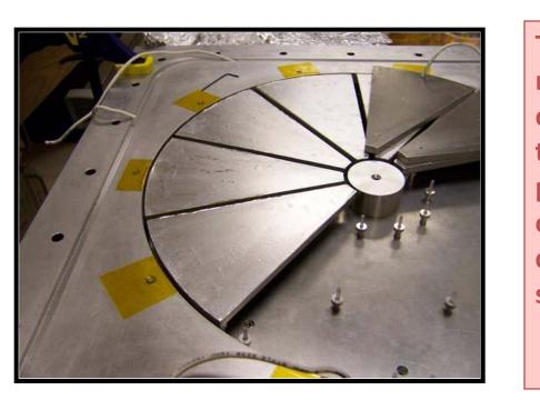
The apparatus used to make RIC measurements included the vacuum chamber, interior of which is shown to the left. Using a combination of a picoammeter and a multiplexer, data could be taken simultaneously on 10 different large area, thin polymer samples.
