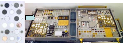
SUSpECS I, II & III: Individual investigators prepared separate sample holders. Holders were integrated into Passive Experiment Containers (PECs). The PEC's were mounted on ISS for 6-12 months stay by astronauts Bob Behnken on EVA 5 March 22nd 2008 with the help of a hammer.
