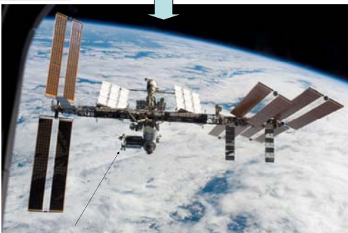
SUSpECS I, II & III: Individual investigators prepared separate sample holders. Holders were integrated into Passive Experiment Containers (PECs). The PEC's were mounted on ISS for 6-12 months stay by astronauts Bob Behnken on EVA 5 March 22nd 2008 with the help of a hammer.
