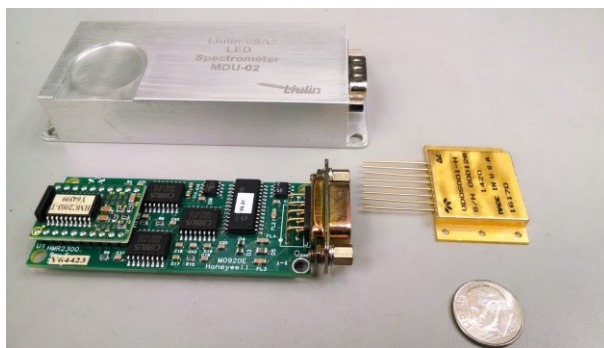
Figure 1: The R3S instrument consists of three commercially available sensors; The Liulin-6SA2 Linear Energy Transfer (LET) spectrometer, a Teledyne \mu Dosimeter TID detector, and a Honeywell HMR2300 magnetometer
