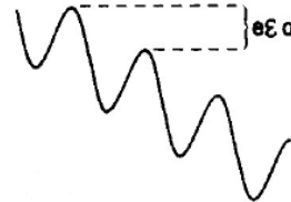
Fig. 3. Application of an electric field enhances the hopping conductivity by lowering the amount of energy need to move between trap sites.
