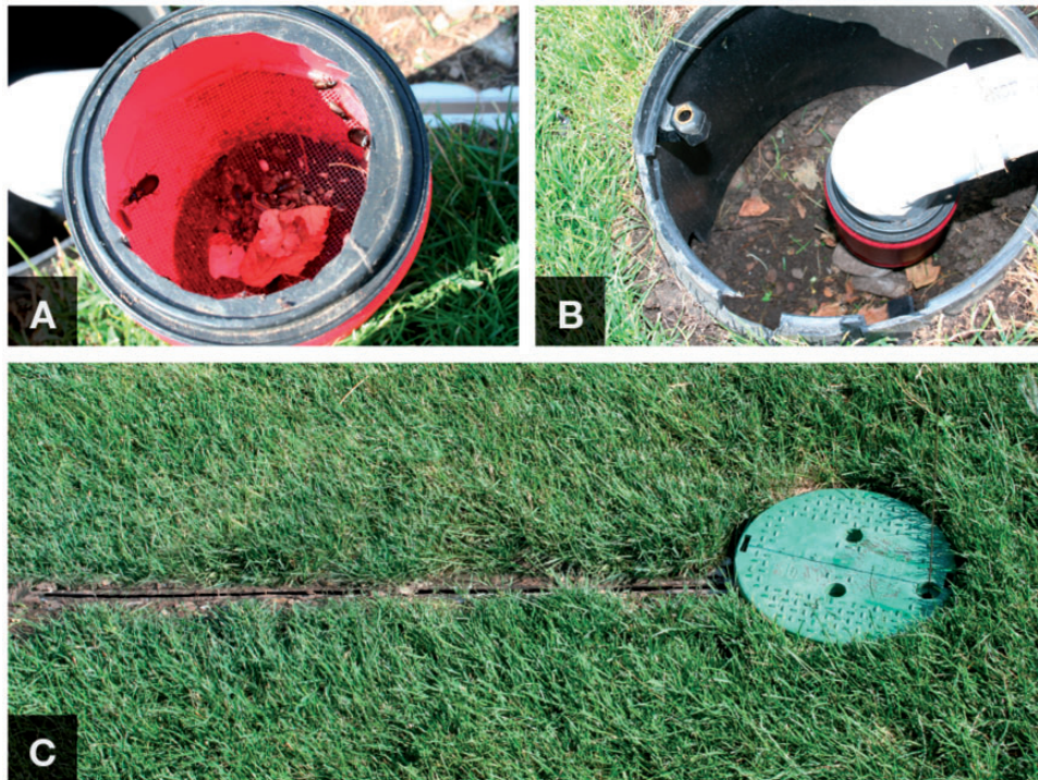
Fig. 5. A linear pitfall trap (similar to Lawrence 1982) is a useful tool for monitoring ground-active adult billbugs. The trap consists of (A) a collection vessel, here made from a recycled coffee container, with a hole cut in the lid for attachment to the end of the PVC pipe. Modifications to the collection vessel can be made including drilling small holes into the bottom for drainage and attaching mesh midway with adhesive to reduce moisture contact with captured insects. (B) The collection vessel attaches to an elbow end of the pitfall PVC pipe and is housed within an irrigation box. The entire trap (C) consists of a 5.08-cm (2 in)-diameter, 1-m (3.28 ft)-long PVC pipe with a 1-cm (0.393 in) slit running the length of the pipe. The pipe is dug into the ground with the slit facing upward so that the slit is flush with the surface of the ground. The other end of the PVC pipe is capped. Photo credits: Madeleine Dupuy, Utah State University.
