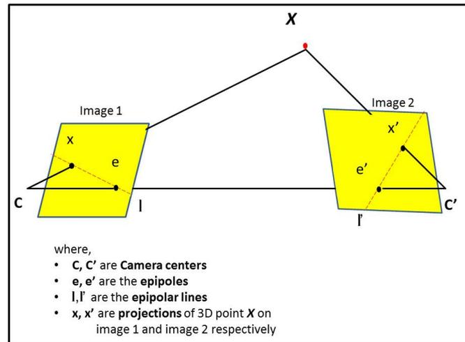
Fig. 3.4: Epipolar geometry.
