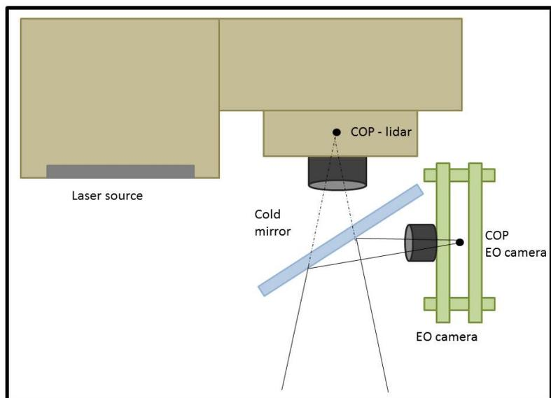
Fig. 2.2: Top view of texel camera without baffle.
