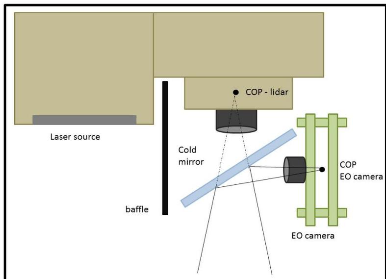
Fig. 2.3: Top view of texel camera with baffle.
