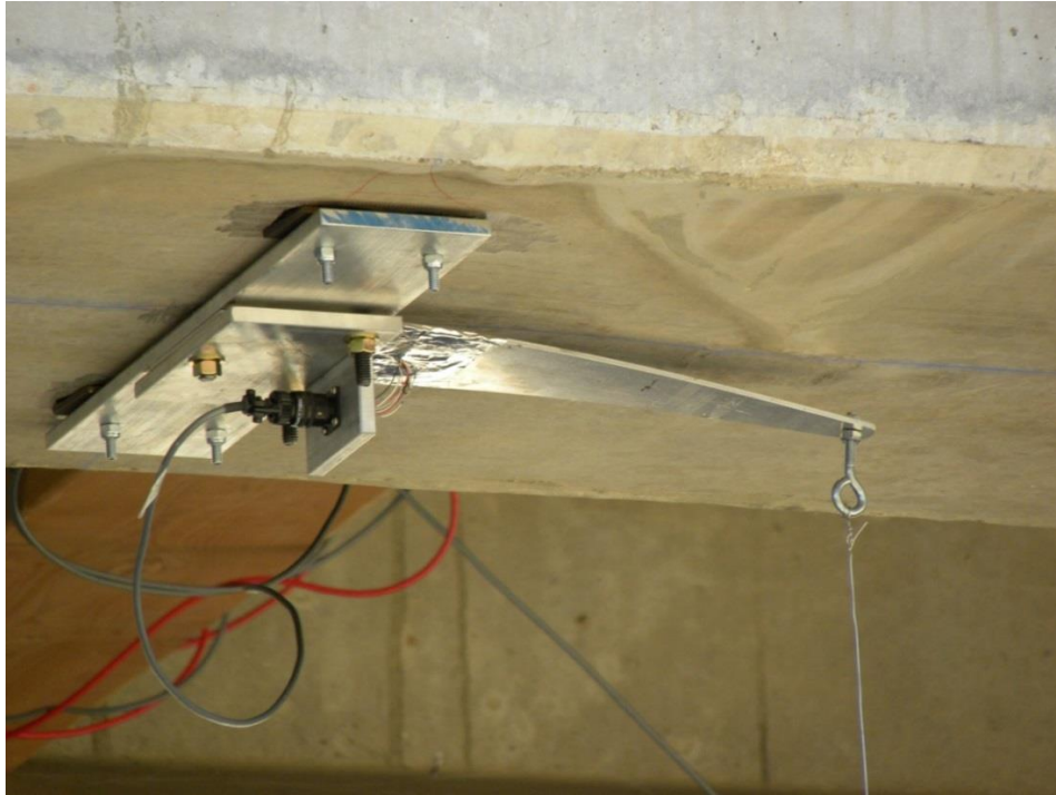
Fig. 6 Deflection instrument, "deflectometer"
