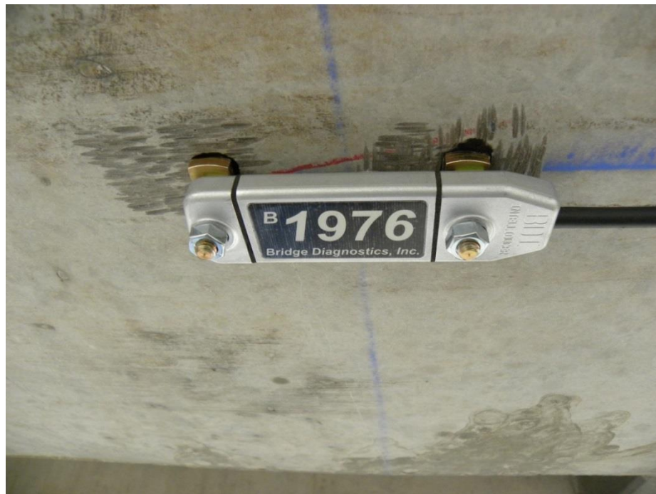
Fig. 5 Surface mounted strain transducer
