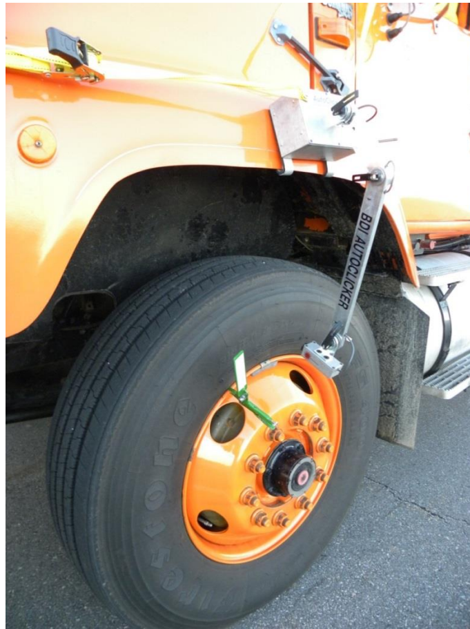
Fig. 20 Automated position tracking sensor, “Autoclicker,” mounted on left front tire of Truck A
