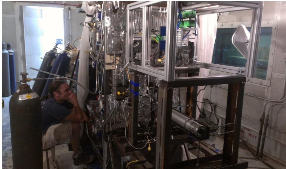
Fig. 5.6: Mobile Nitrous oxide Supply and Test Resource cart.
