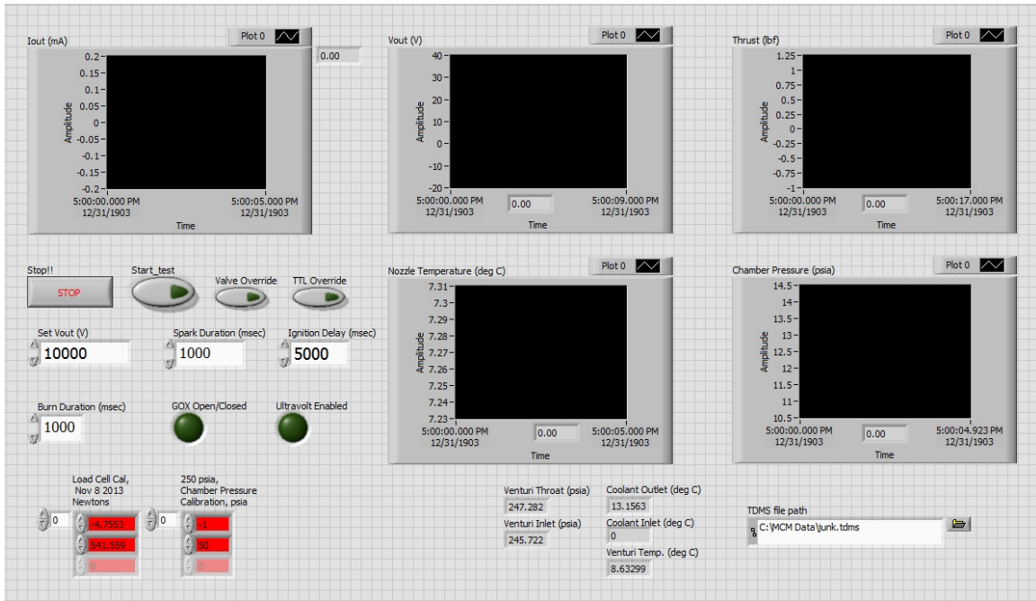
Fig. 5.8: Operator’s graphical interface for ABS arc igniter testing.
