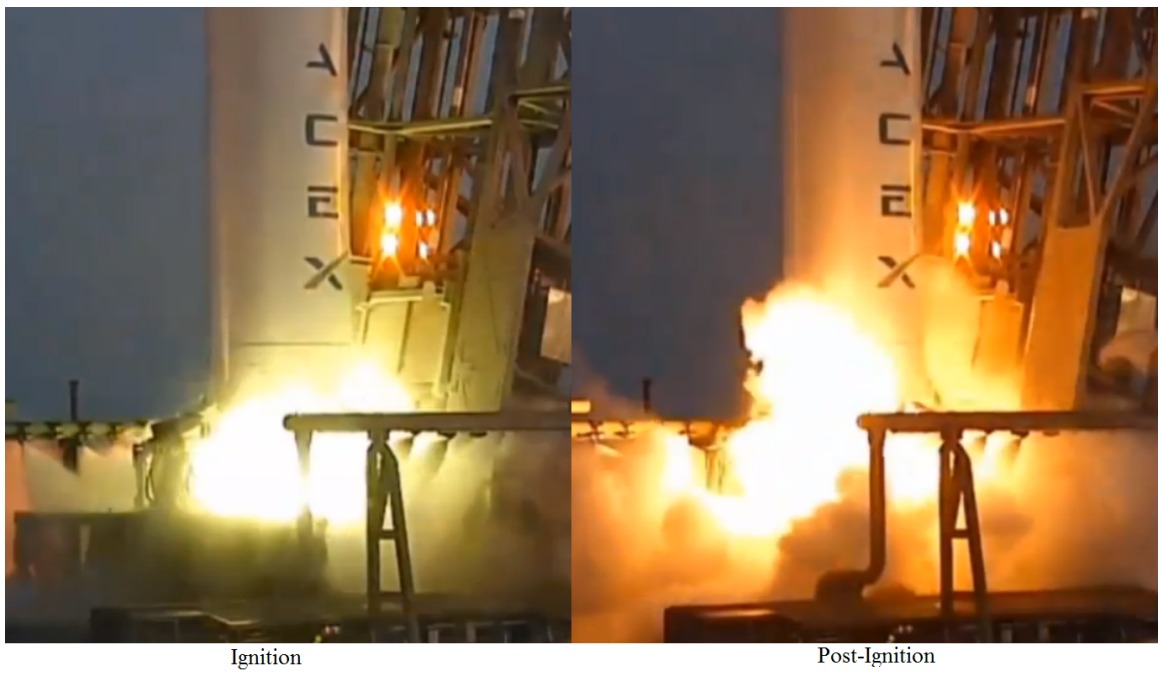
Fig. 2.4: Comparison of Merlin 1D flame color during and after TEA-TEB injection.
