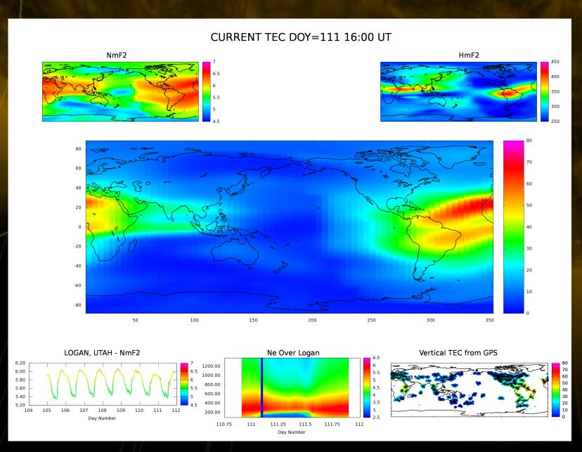
The Gauss-Markov Kalman filter is based on a physics based model of the ionosphere and a Kalman filter data assimilation algorithm. The USU-GM is a global model that can support regional, higher-definition assimilation windows within the model specification. The regional higher-definition window is used in areas where there is a large amount of data. The current version of the model is GAIM-GM2.9.0,
