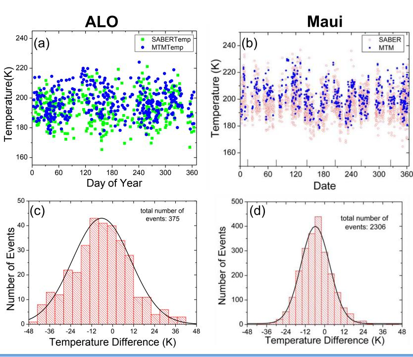
Time series plots for only the closest overpass SABER Temperatures (green) and the MTM OH Temperatures (blue) (a) for 2009-2013 at ALO are compared with overpass data for 2003 at Maui (b) showing SABER (red circles) and MTM (blue) temperatures (Note: Maui comparison used a 10°x20° box). The histogram plots (c) and (d) with fitted Gaussian curves show the distribution of the differences in the MTM and SABER measurements. Both indicate SABER temperatures are ~5 K lower than MTM temperatures.
