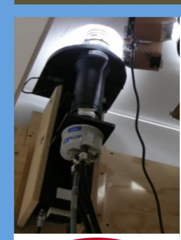
The USU CEDAR MTM is a high performance CCD imaging system designed to provide accurate measurements of mesospheric temperature variability and gravity wave intensity and rotational temperature perturbations using observations of the OH (6,2) band airglow emissions at a nominal altitude of ~87 km.
