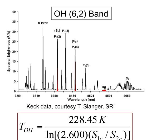
•OH transition parameters from Goldman et al., 1998. •Relative band intensity from (S<sub>1c</sub>+S<sub>2c</sub>) and T using simplified LTE calculation.
