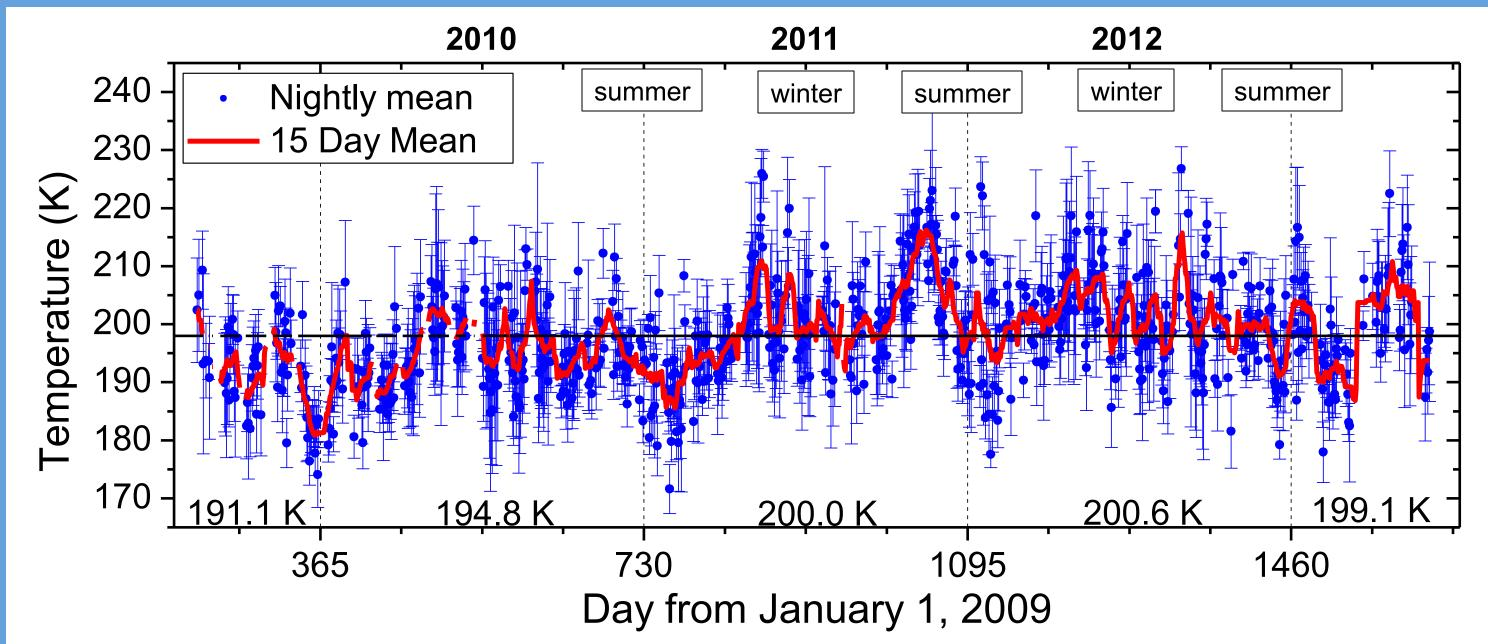
MTM nightly averaged OH temperature measurements from August 12, 2009 until June 5, 2013. Days are counted from January 1, 2009, where years are separated by black vertical lines. The blue circles are the nocturnal mean temperature and the error bars represent the standard deviation in temperature each night. A 15 day running average (red line) and the mean temperature of 198 K (black) are shown.
