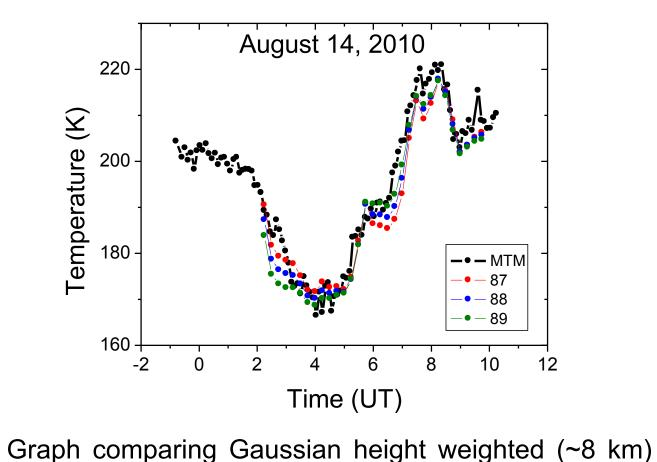
MTM OH temperature measurements with coincident University of Illinois Na wind-temperature lidar observations from ALO. Note high quality of the agreement using these two different techniques. [Courtesy G Swenson, A. Liu, and Y. Zhao]
