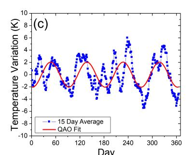
15 day running-average OH temperature data from ALO (2009-2012) fit to (a) an annual, (b) a semi-annual, and (c) an unusual ~90 day (quarter-annual) oscillation. ALO temperature amplitudes are compared to Maui results, which used the below fit, are shown in the table (courtesy Y. Zhao).
