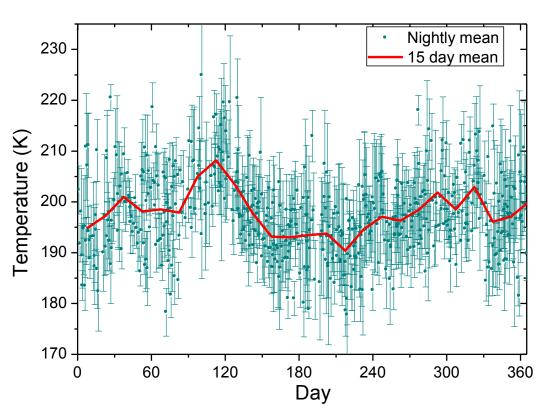
ALO MTM nightly mean OH temperature (blue) folded into one year. As above, the error bars represent the nightly standard deviation and the red line is a 15 day running average. Similar data is shown from three folded years of data from the Maui-MALT campaign (teal).
