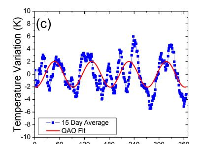
15 day running-average OH temperature data from ALO (2009-2012) fit to (a) an annual, (b) a semi-annual, and (c) an unusual ~90 day (quarter-annual) oscillation. ALO temperature amplitudes are compared to Maui results, which used the below fit, are shown in the table (courtesy Y. Zhao).
