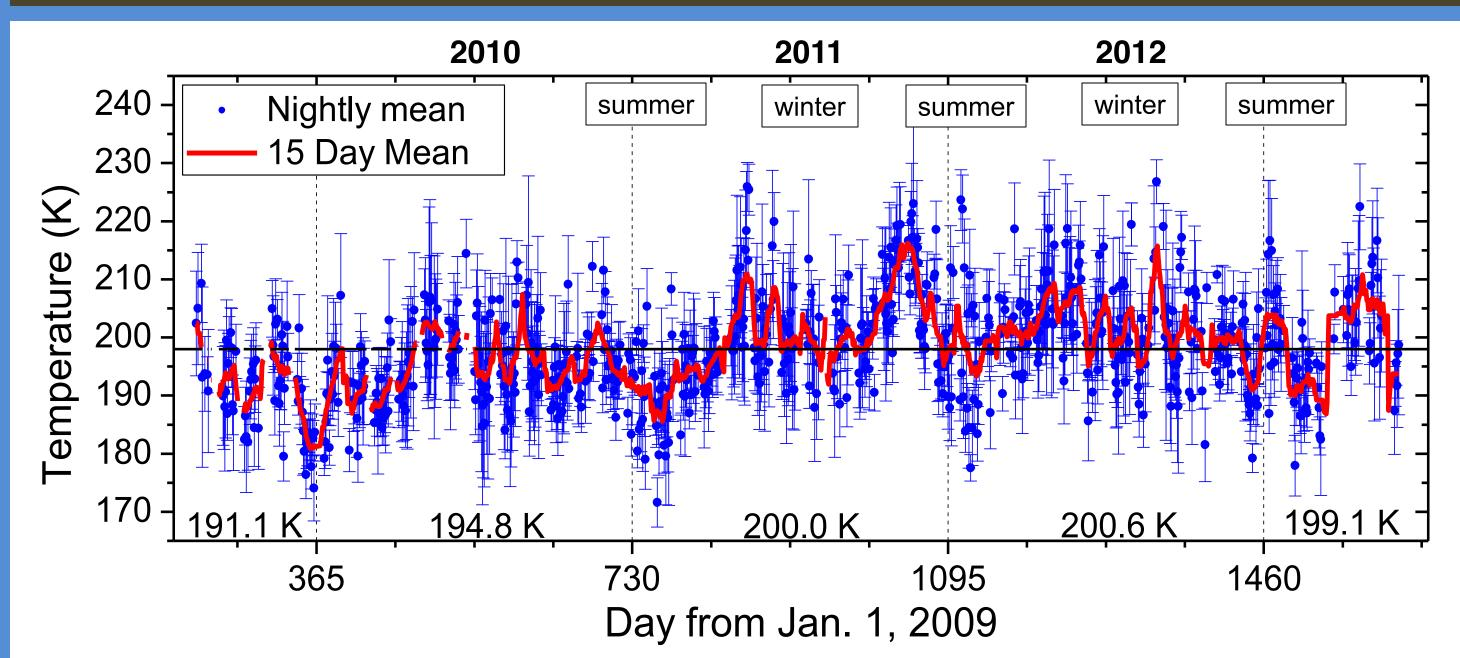
MTM nightly averaged OH temperature measurements from August 12, 2009 until June 5, 2013. Days are counted from January 1, 2009, where years are separated by black vertical lines. The blue circles are the nocturnal mean temperature and the error bars represent the standard deviation in temperature each night. A 15 day running average (red line) and the mean temperature of 198 K (black) are shown.
