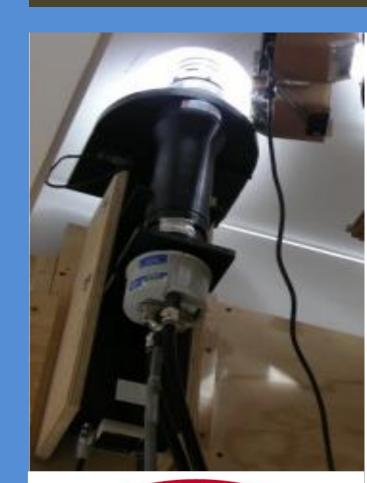
The USU CEDAR MTM is a high performance CCD imaging system designed to provide accurate measurements of mesospheric temperature variability and gravity wave intensity and rotational temperature perturbations using observations of the OH (6,2) band airglow emissions at a nominal altitude of ~87 km.
