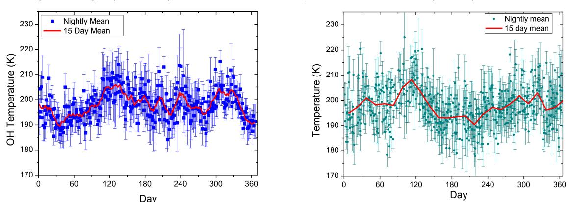
ALO MTM nightly mean OH temperature (blue) folded into one year. As above, the error bars represent the nightly standard deviation and the red line is a 15 day running average. Similar data is shown from three folded years of data from the Maui-MALT campaign (teal).
