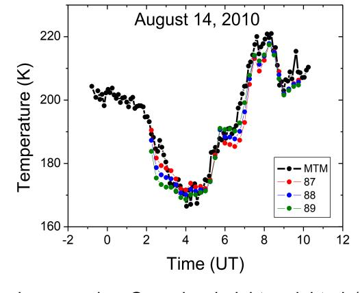
Graph comparing Gaussian height weighted (~8 km) MTM OH temperature measurements with coincident University of Illinois Na wind-temperature lidar observations from ALO. Note high quality of the agreement using these two different techniques. [Courtesy G Swenson, A. Liu, and Y. Zhao]
