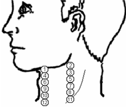
Figure 1 Accelerometer placement locations for neck location testing (image courtesy U.S. Army Research Lab Human Research & Engineering Directorate).
