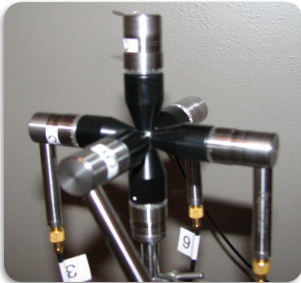
Figure 2: A six-microphone energy density probe. This probe enables two plane's of measurements to be made.
