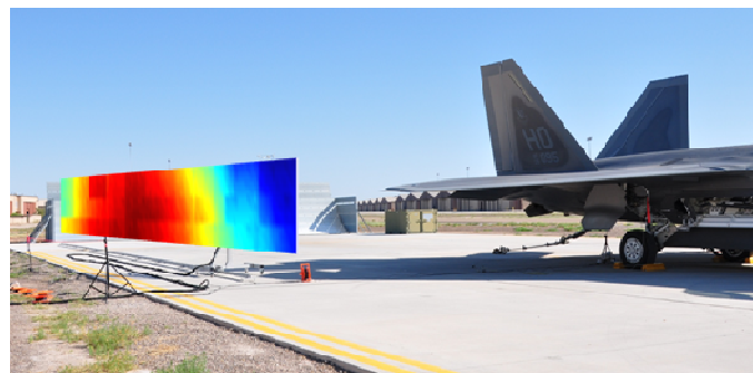
Figure 3 An example sound pressure level map overlaid with the jet photo at the approximate measurement location.
