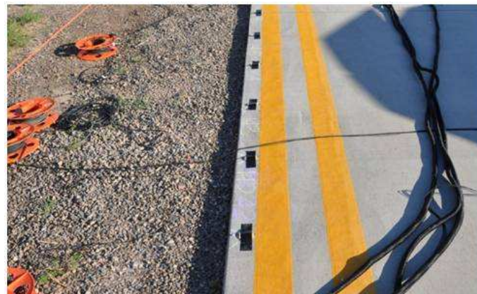
Figure 4 Fifty reference microphones were placed on the ground 12 m from the jet centerline, which measured sound pressures simultaneously with each scan.
