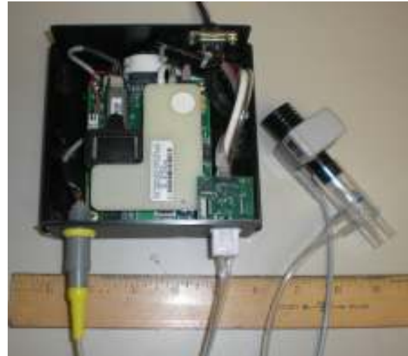
Figure 3 The prototype critical care system circuitry and sensors. The proposed study would modify the gas flow sensor and algorithms to facilitate exercise testing
