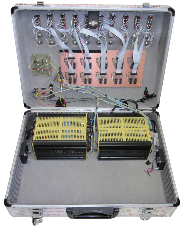
Fig. 5. Inside View of Amplifier Box
