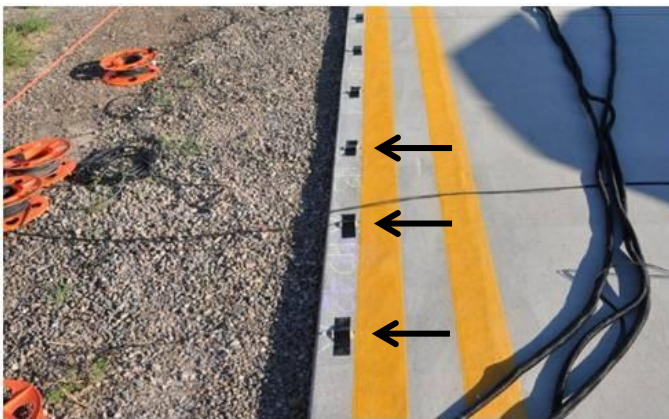
Figure 4 Fifty reference microphones were placed on the ground 12 m from the jet centerline, which measured sound pressures simultaneously with each scan.
