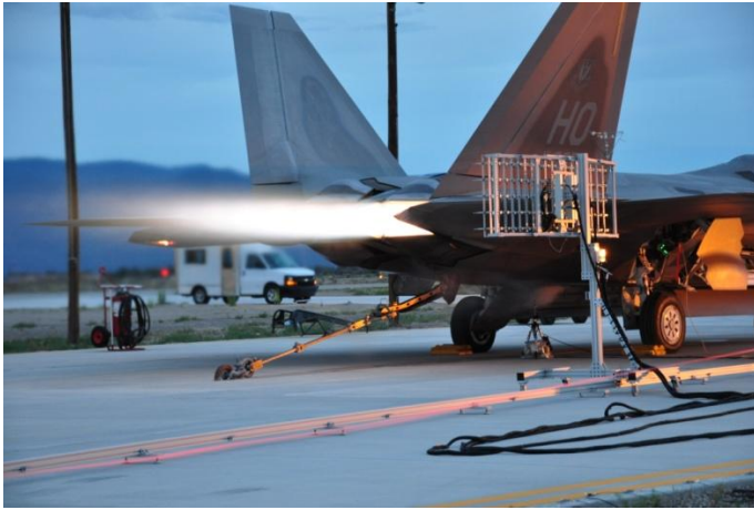
Figure 2 Blue Ridge Research and Consulting 90-microphone array, scanning the near field of the jet on an F-22 Raptor.
