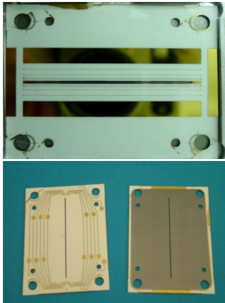
Figure 2 Finished ceramic plate (top) without germanium and (bottom) with germanium and the back side for electrical contact from a PCB.
