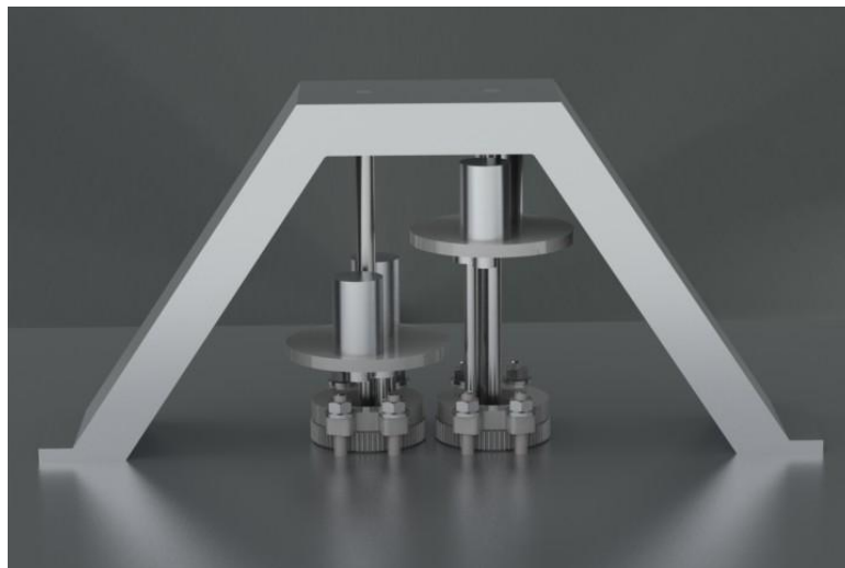
Figure 4. Motors are located above the mechanism at a location safe from water, oil, etc.
