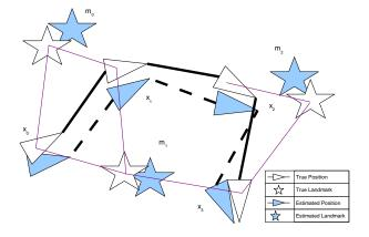
Figure 1. SLAM Problem Diagram: The true states and landmark positions are shown in white triangles and stars respectively. The measured states and landmarks positions are shown as blue arrows and stars respectively.
