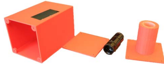
Figure 17: Mock-up 3D Print with Lens and Solar Cell
