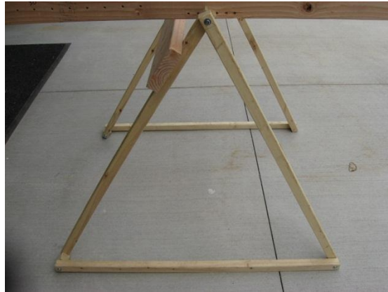
Figure 10. Completed triangular stand assembly.
