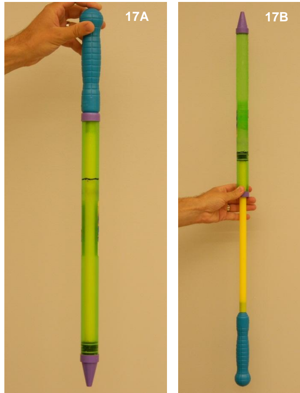
Figures 17A-17B. The water blast tube, with its 185 mL water level marked (17A) and filled with water to the mark (17B).
