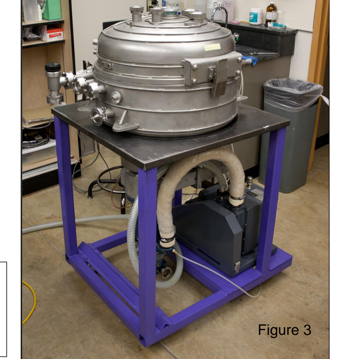
Figure 3. finished vacuum system
