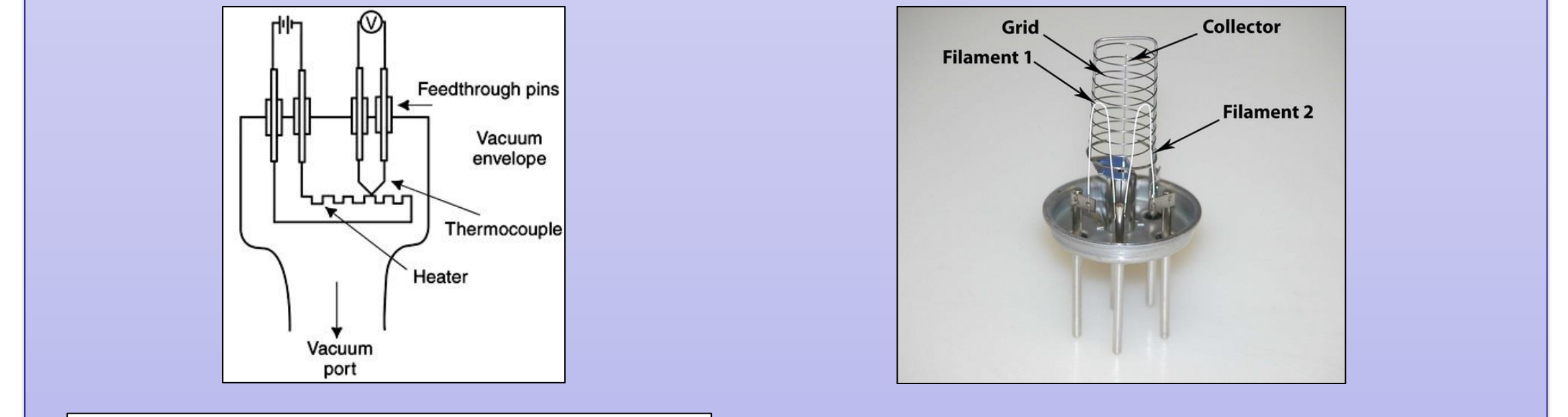
Figure 12. Thermocouple gauges operate on the principal of thermal conductivity. In lower pressures there are fewer molecules to absorb thermal energy. Temperature is measured and calibrated to read pressure as a product of molecular density. Thermocouple gauges operate in higher medium vacuum ranges.
