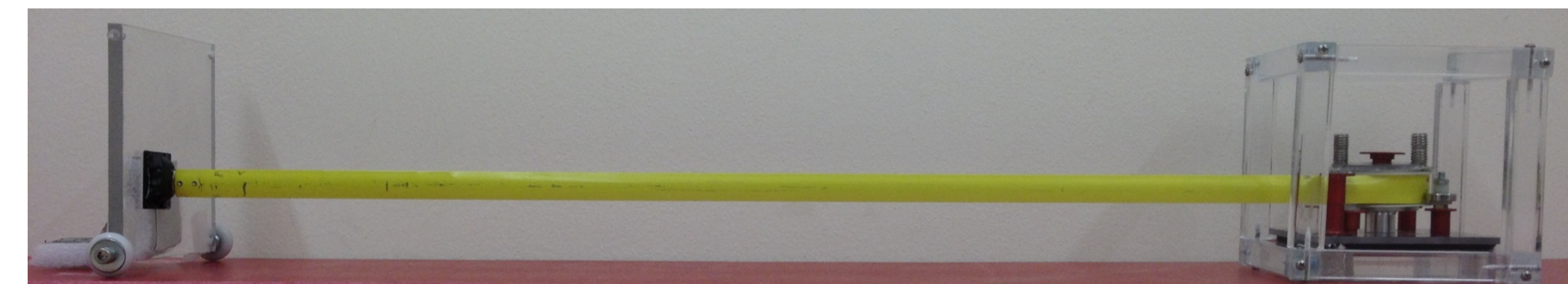
Figure 2- Prototype 1 demonstrating the use of spring steel for .5 meter boom deployment
