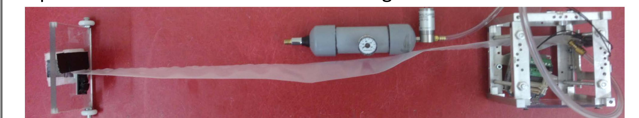
Figure 4- Prototype 1 of gas actuated inflatable boom deployment system
