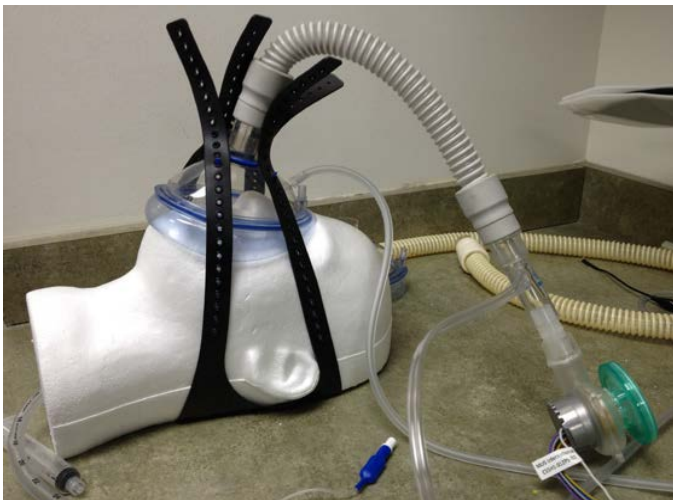
Figure 3: Prototype blower and face mask to deliver rescue breathing during CPR.
