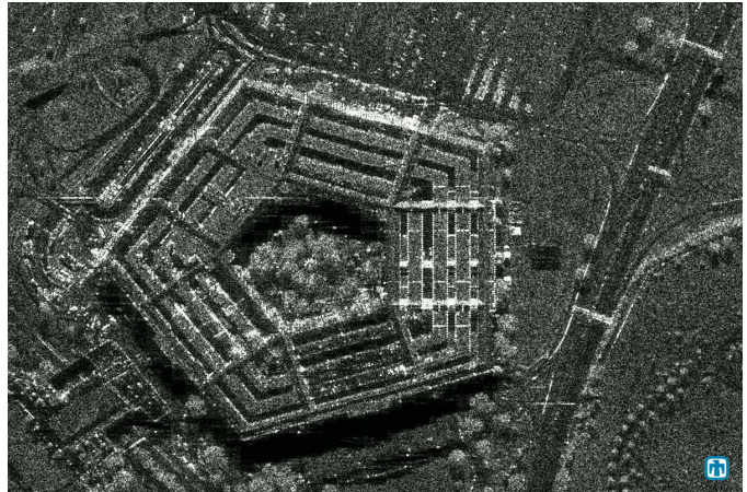
Fig. 1. Ku-band SAR image of the Pentagon in Washington, D.C. (Courtesy Sandia National Laboratories).
