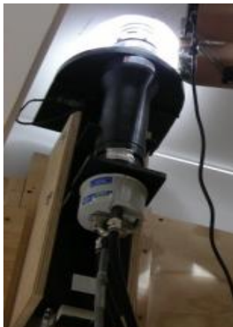
Figure 2. Picture of all-sky imaging system. Fish eye lens at top, followed by filter wheel. CCD imager and cooling system are positioned at bottom.
