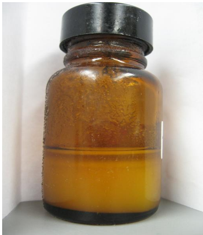
Figure E1. Separation of liquid and crystals in non-sonicated IESBO stored at 25 °C.
