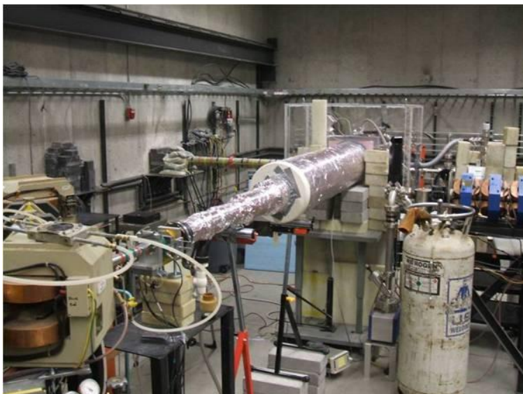
FIG. 3.11. The IAC beam line configuration showing (left to right) accelerator, beam shutter assembly, He-filled drift tube, cryogenic enclosure, sample window, and RIC chamber.
