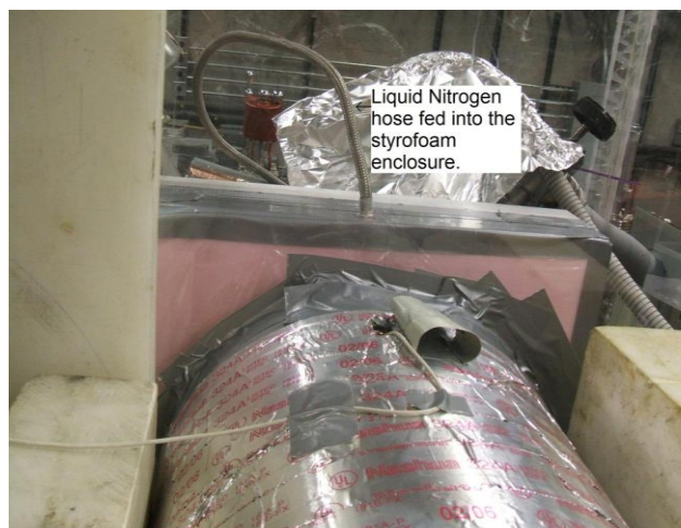
FIG. 3.16. Cryogenic setup at IAC showing the liquid nitrogen hose fed into the styrofoam insulation.
