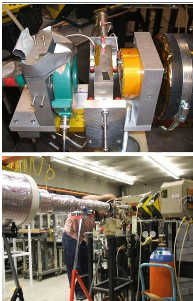
Fig. 3.10. RIC shutter assembly. (Above) Beam restricting shutter assembly and aluminum pickup coil (shown in blue) used to measure beam current. (Below) Shutter assembly located between LINAC aperture and the drift tube.
