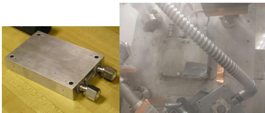
FIG. 3.13. Cryogenic temperature reservoir (left). Two reservoirs connected in series on the back of the RIC chamber (right).
