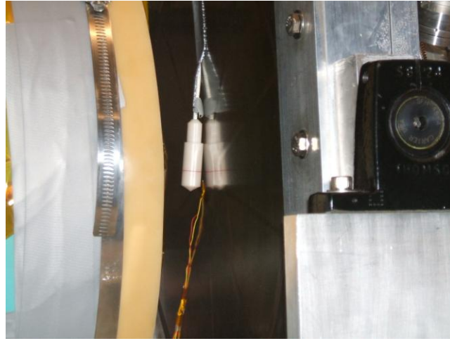
FIG. 3.17. Miniature ionization chamber positioned between the RIC chamber window and the drift tube.
