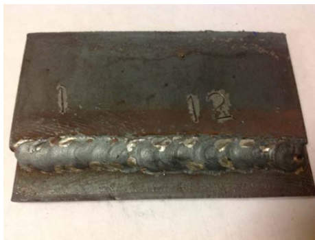
Figure 5. GMAW weld test coupon.
