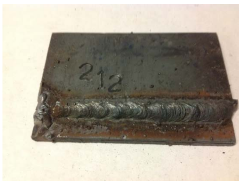
Figure 6. SMAW weld test coupon.
