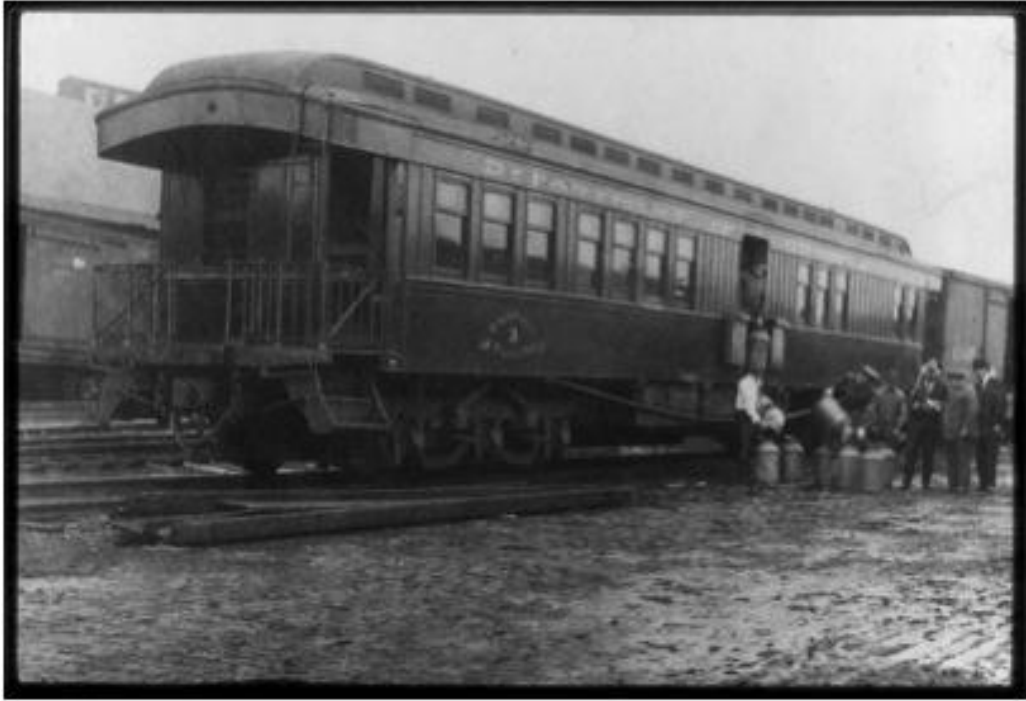
Figure 7. “Aquarium” railcar designed to transport fish fry. U.S. Department of Commerce. Photo courtesy of AndersHalverson.com
