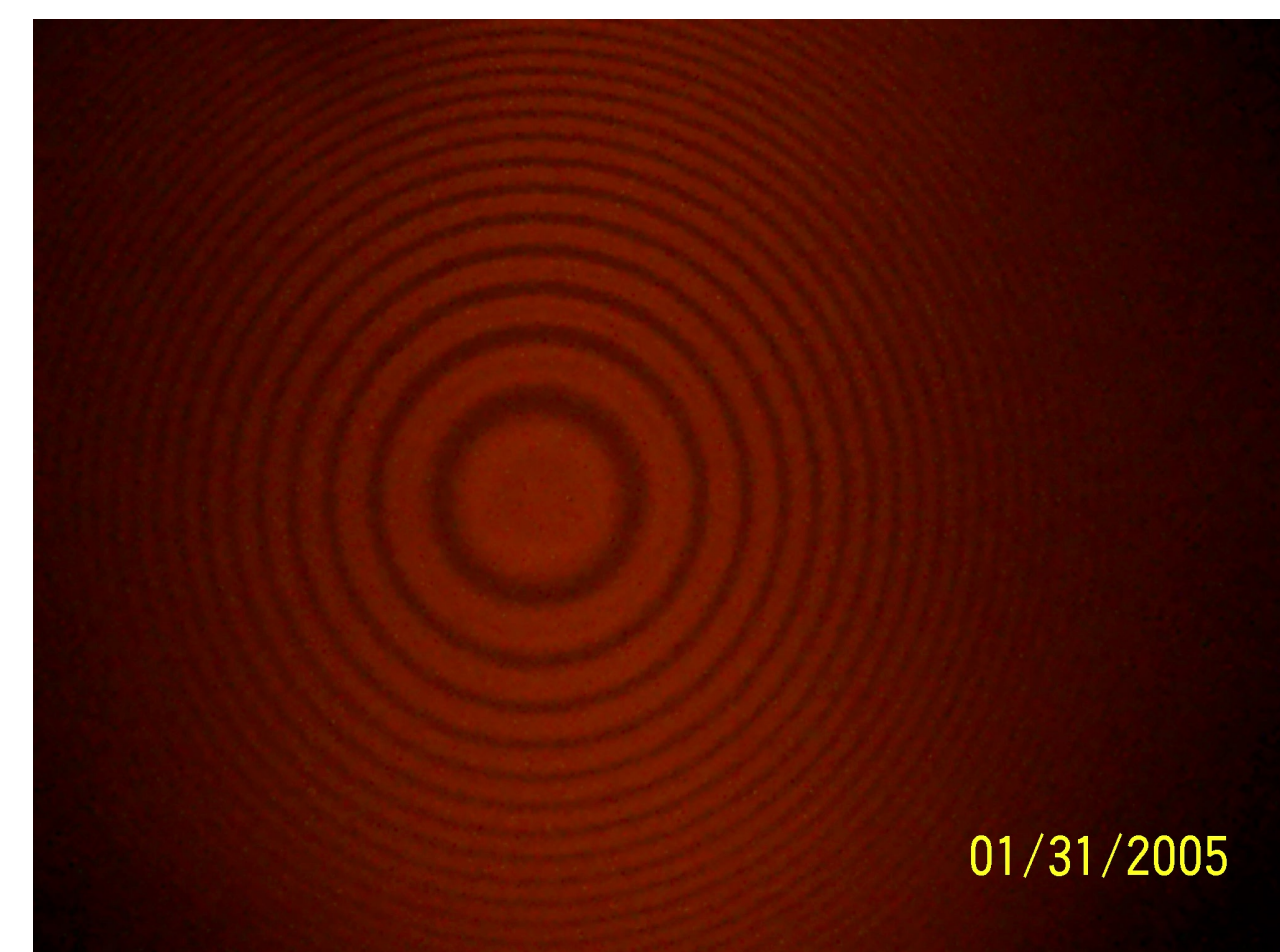
Figure 4. Example of an interference pattern from a FPI.
